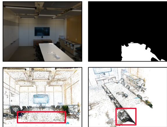
Figure 4. A failure case of SAGA. The upper-right part shows the segmentation result, and the lower part shows the mean of Gaussians of the 3DGS model. The failure is caused by the incorrect geometric structure of the learned Gaussians by 3DGS.
